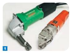
Electric shears and electric nibblers are power tools useful for cutting steel building frames. They provide an alternative cutting method to hand tools such as snips.
