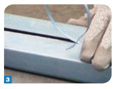
The **electric shear** operates by cutting-out a continuous strip that leaves the material on either side of the cut undistorted.
