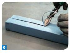
Cutting with a shear will produce a strip of scrap that can easily and safely be disposed of in a scrap recycling container.
