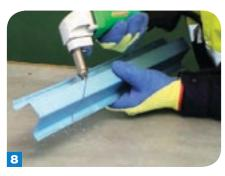
Like the shear, the nibbler will cut in a straight line. It will also cut other steel framing profiles such as roof battens.
