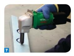
The **electric nibbler** is more versatile than the shear giving you scope to cut to a particular shape.
