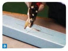
Left cut snips (red) allow you to cut in a curved direction to the left. Right cut snips (green) allow you to cut in a curved direction to the right.
