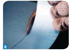
Both left (red) and right (green) snips allow you to cut in a straight line. Mark your line with a marker and ruler before cutting.
