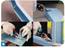
Be careful not to damage the snips if the section you are cutting cannot easily be peeled away.
