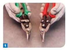
We recommend using left-offset and right-offset aviation snips. The term 'offset' refers to the blade being offset to the handle – allowing you to work above the material being cut. The red handled snip is the left cut snip. The green handled snip is the right cut snip.
