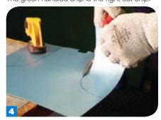
When cutting with snips, make sure the scrap is peeled away. This will make it easier on the blades and will make it easier for you to accurately guide the snips.
