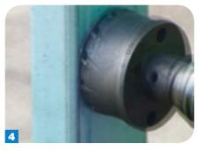
Using the pilot hole, drill back from the other side to complete the hole.
