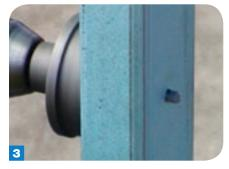
Once the first side is penetrated, push through to locate the pilot hole on the other side.
