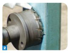
Use a lubricant to assist with cutting and extend the life of the cutter.
