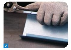
Using your left or right offset snip, notch out the return lips. These are small sections and will peel away easily.
