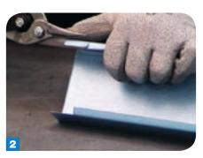
Using your left or right offset snip, notch out the return lips. These are small sections and will peel away easily.
