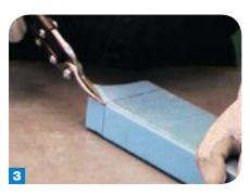
Use the left cut snips to cut in on the corner.
