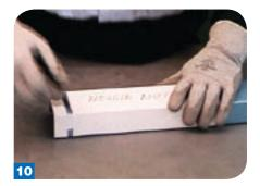
**Using templates.** Use a pre-made template to mark out the notch and fold lines. A template helps speed up the process and makes the job of cutting easier.
