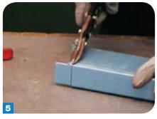
Finally, cut back into the other corner to finish the notch.
