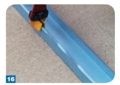
Using this tool you only have to mark the location of the stud then flatten the lips of the base plates, insert the stud and the job's done ready for fixing.
